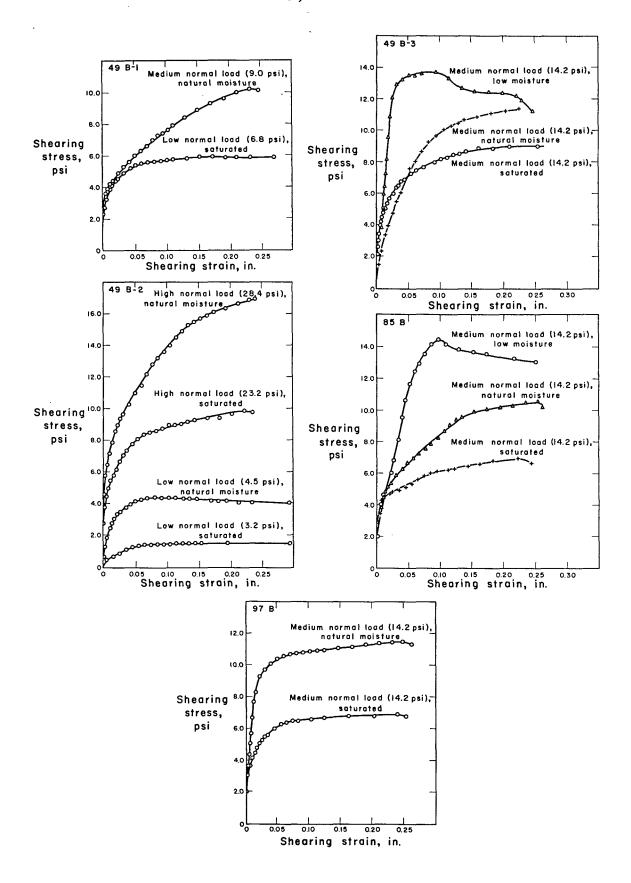
value rather than the maximum value is entered on the plot there is no sharp increase in strength. This decrease in shearing strength with increasing strain also occurs under certain conditions in other soils.
