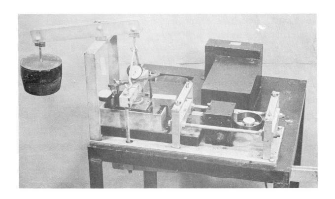
consolidation became so slow that further consolidation would be negligible (less than about 0.0003 inches per hour), a final reading was recorded on the data sheet. The time required was two hours or less for light loads and from four to six hours for the heavy loads.
